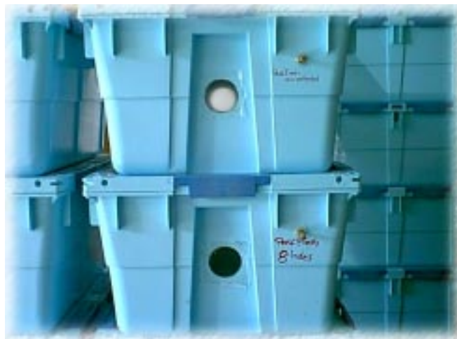
Figure 1. Modified SLX containers showing sealed MAP film patches at forward and rear locations.
